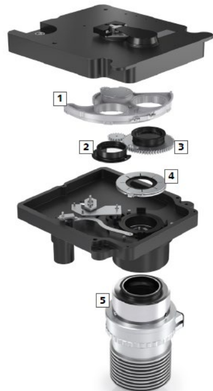
The Axioscan 7 brightfield imaging performance is driven by a motorized condenser and a powerful white light source: 1) Motorized modulator disc 2) Circular polarizer 3) Motorized linear polarizer 4) Motorized aperture diaphragm 5) White light LED light source
